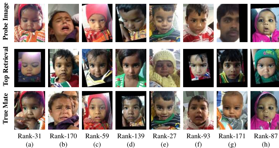
Figure 17: Example face retrieval results. All examples shown are retrieval errors made by COTS-B against a gallery of 185 face images (21 out of 206 face images failed to enroll). Errors are due to variations in pose, illumination, and expression. In probe image (g), a background adult face was enrolled, rather than the foreground face of the child.
