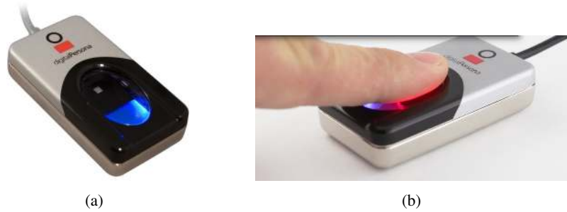
Figure 5: (a) The 500 ppi Digital Persona U.are.U 4500 HD fingerprint reader [18] used to collect child fingerprints. The approximate reader size is 65 mm x 36 mm x 15.56 mm and it weighs 105 grams. (b) A red light glows once the finger is placed on the reader platen to trigger the fingerprint image capture.
