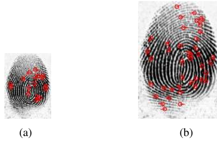
Figure 6: Extracted minutiae marked on (a) the original fingerprint image (17 minutiae were extracted), and (b) the upsampled fingerprint image (51 minutiae were extracted) of a 7 months-old child using the tenprint SDK (COTS-T).
