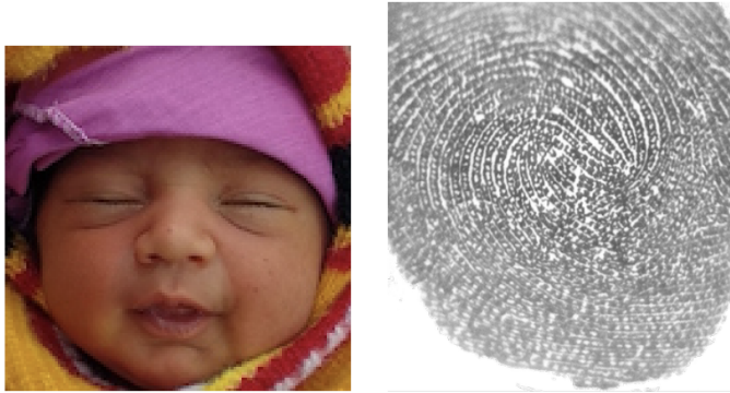
Fig. 12: Face image and corresponding thumb-print of a 1-week old infant [52]. The thumb-print was captured and matched using a custom 1,900 ppi reader and accompanying high-resolution matcher, since the standard 500 ppi COTS readers and matchers do not have sufficient resolution to capture and match an infant’s fingerprints.
