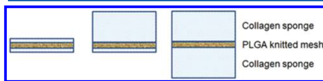
Figure 9. Schematic illustration of three structural designs of PLGA/collagen hybrid scaffolds. Black, PLGA knitted mesh; gray, collagen type I sponge. Modified with permission from ref 232. Copyright 2010 Elsevier Ltd.
