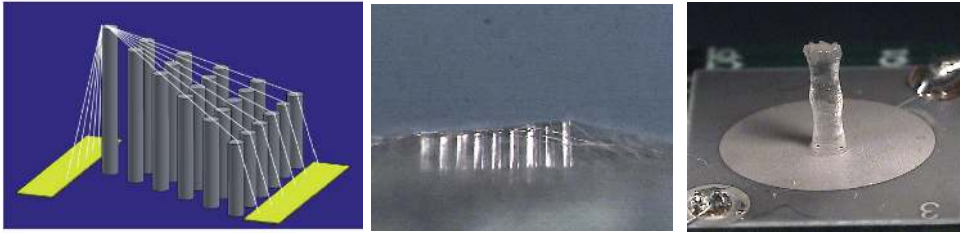
Figure 12: MEMS sensors emulating advanced biomimetic features. (Left) Hair cell-inspired NEMS sensor; a schematic showing 6 rows of PDMS polymer pillars of graded height (maximum height 425 microns). The links connecting the distal tips of the pillars are formed by polyvinylidene fluoride polymer that generates electric charges as the pillars bend causing stretching in the fibers, amplifying the signal. (Center) Photo of the implemented NEMS sensor. (right) Stereolithography fabricated whisker-like sensor on a piezoelectric diaphragm (whisker height 3 mm) (Kottapalli et al. 2014b).
