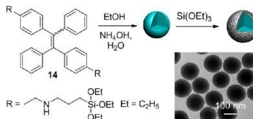
FIGURE 12. Fabrication of 14 -cored FSDs and their TEM images.
