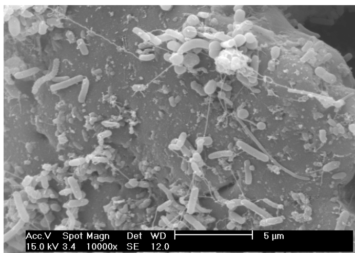
Figure 7.1 ESEM micrographs of SRB colonising the polystyrene surface.
