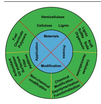
**Fig. 4** Schematic representation of the main processes for lignin extraction and possible chemical modifications performed in order to valorize lignin, depending on the applications [66]
