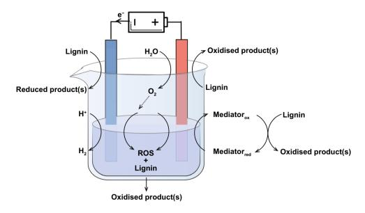
Fig. 7 Electrochemical lignin valorization. Electro-oxidation at the anode via direct, mediated methods and via the generation of reactive oxygen species (ROS) from reduction of  $O_2$ . Electroreduction via direct method. Water splitting competes with lignin electrochemical conversion at both anode (OER) and cathode (HER)
