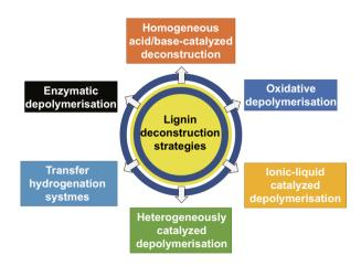
Fig. 5 Schematic diagram of the deconstruction strategy of lignin [81]
