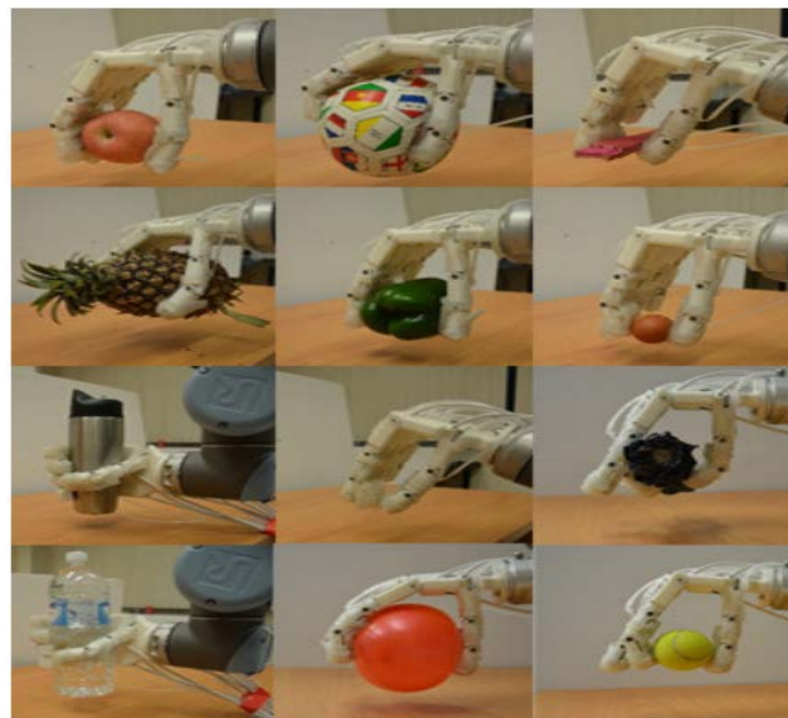
Figure 6. This shows the teleoperated bimanual assembly carrying a large assortment of different shapes and sizes to show how well it can grip with its soft layer and cumulative hand strength (Reprinted with permission from Zhu, G. et al. [36]. Copyright 2020, CC BY 4.0 International).
