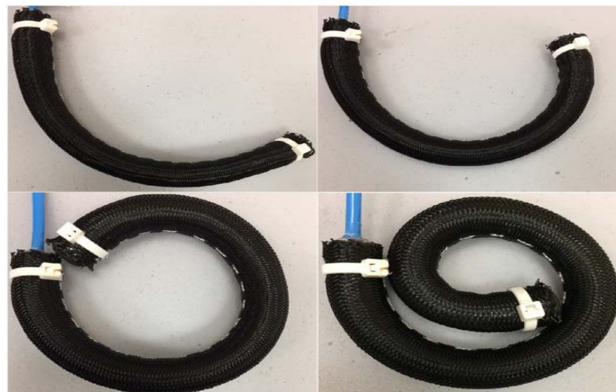
Figure 15. EBPAM pressurized under different amounts of pressure; increasing from top-left to bottom-right (Reprinted with permission from Al-Fahaam, H., et al. [112]. Copyright (2018), with permission from Elsevier).
