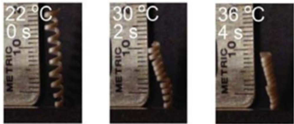
Figure 16. A simple TFAM experiencing thermal actuation (Reprinted with permission from Leng, X., et al. [26] Copyright 2020, CC BY NC ND 4.0 International).
