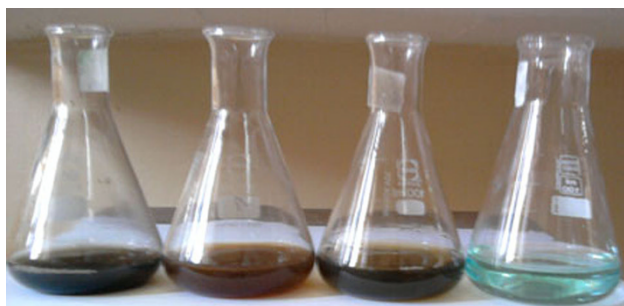
Fig. 1 Color change during the phyto-reduction of \text{CuSO}_4 into CONPs at the beginning and after 48 h of reaction
