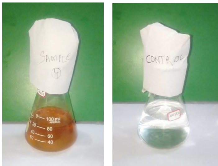
Figure 2. Colour change of reaction mixture from transparent to brown, indicating the biosynthesis of silver nanoparticles after incubation (Shukla and Sandhu 2017).
