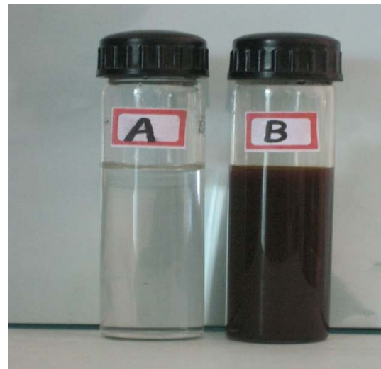
Fig. 1 A Silver nitrate ( \text{AgNO}_3 ) solution and B color change during the reduction of \text{AgNO}_3 into AgNPs by the extract of S. wightii after 24 h of incubation
