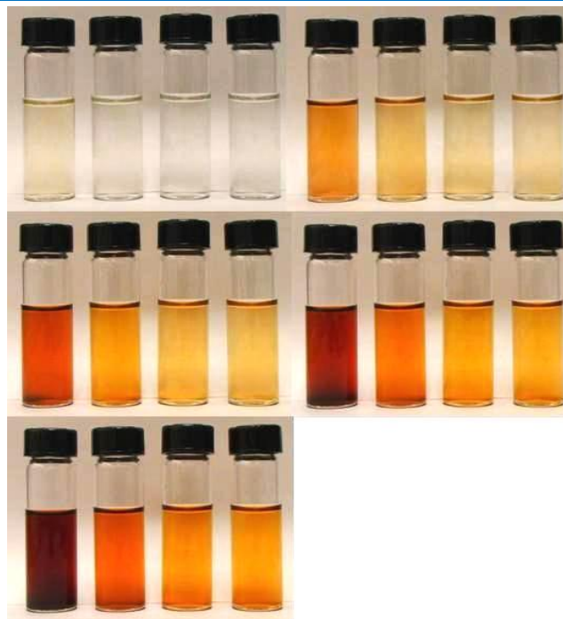
Fig. 4. Photographs of the varying concentrations (A-1:25, B-1:50, C-1:100 and D-1:200) of leaf broth to silver nitrate.
