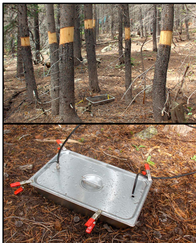
Figure 2. (top) Trenched experimental plot with girdled trees and stainless steel collar placed into the soil. (bottom) Soil chamber during the measurement of BVOCs with an ambient line to quantify ambient BVOCs and a chamber line to quantify soil BVOCs.
