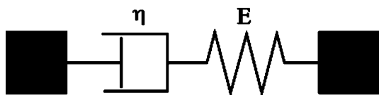
Figure 2. A dashpot (damper) with viscosity \eta in series with a spring of elastic modulus E is the simplest model for a viscoelastic fluid capable of capturing stress relaxation behavior.
