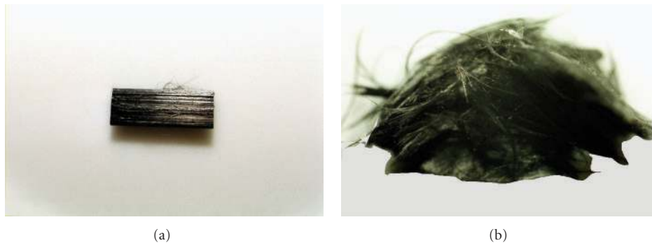
FIGURE 6: (a) Typical composite bar exposed to sulfuric acid, hydrochloric acid, or phosphoric acid. (b) Composite bar exposed to nitric acid over a similar time period then washed and dried.
