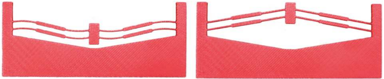
Fig 7. Bistable mechanism prototyped in ABS plastic, using a Dimension SST 1200ES 3D Printer, in its second stable position (left) and its fabricated position (right).
