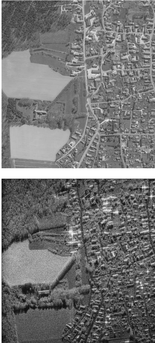
Fig. 8. Optical image (LVG Bayern) and bistatic SAR image (processed by a time-domain algorithm) of Oberndorf, Germany.
