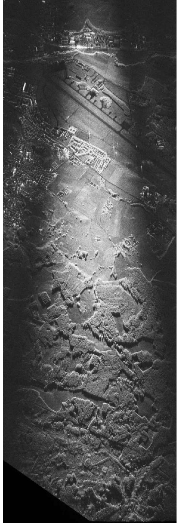
Fig. 13. Bistatic spotlight TerraSAR-X/F-SAR image. 7680 m in ground-range, 2560 m in azimuth. Radar illumination from top.
