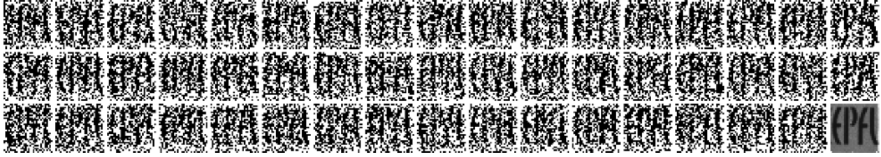
Fig. 9. Reconstructing an image from the binary measurements taken by a SPAD sensor [17], with a spatial resolution of 32 \times 32 pixels. The final image (lower right corner) is obtained by incorporating 4096 consecutive frames, 50 of which are shown in the figure.
