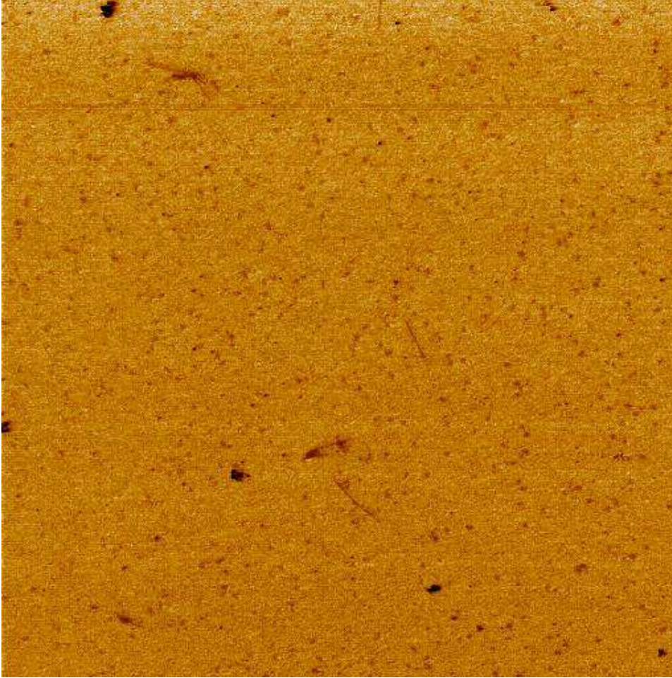
Fig. 7. AFM phase image of bitumen AAA (15 \mu\text{m} x 15 \mu\text{m} ).
