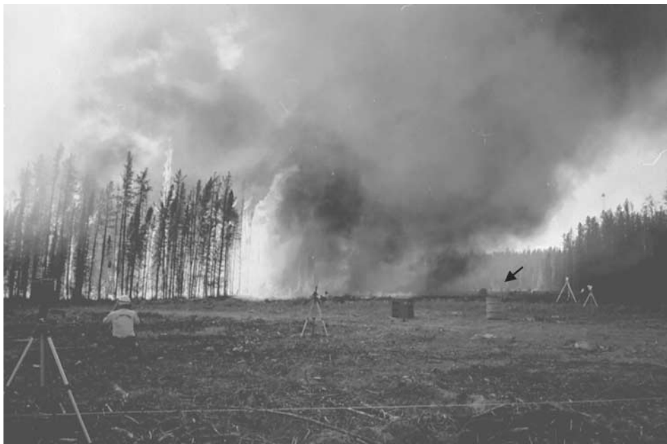
Figure 2. View of the 4 July burn as the flame front reaches the end of the plot and sooty smoke extends through the fireguard. Sampling equipment, located on the right side of the fireguard (arrow), is positioned to collect particles from the black plume near ground level shown in the photograph. See color version of this figure at back of this issue.
