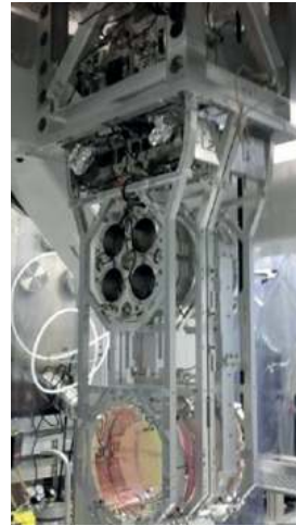
Photograph of one of the first production quadruple suspension systems ready for installation in aLIGO.
