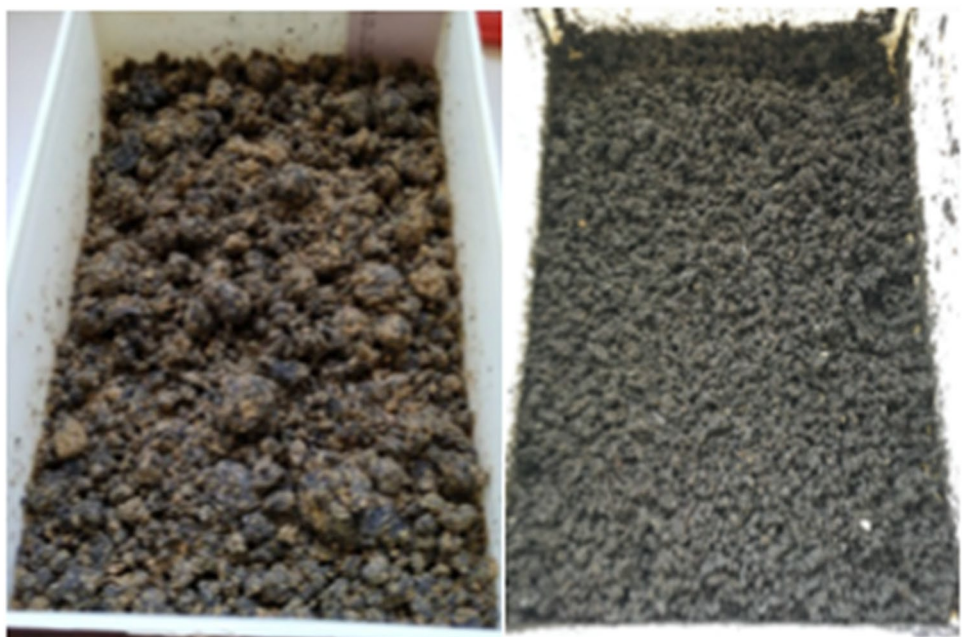
Fig. 4 Feeding substrate S50: before (left) and after 9 days (right) of bioconversion with H. illucens
