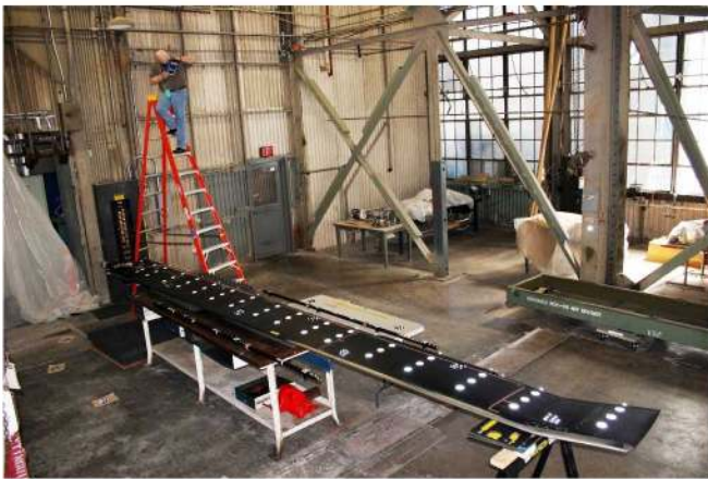
Figure 5. Blade with two-inch diameter retro reflective targets installed.
