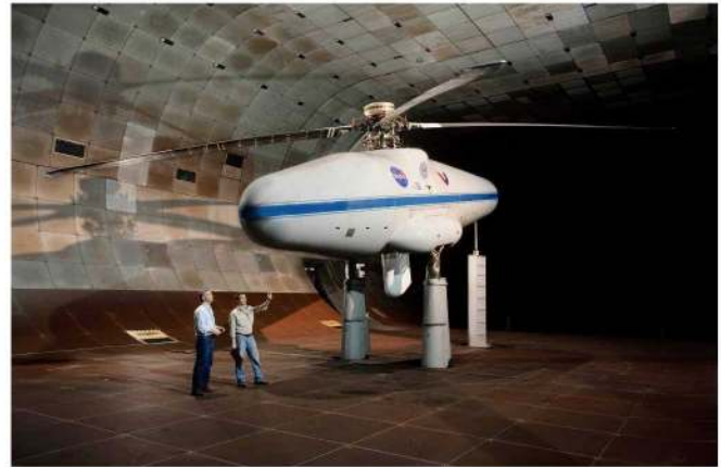
Figure 2. UH-60A installed on the LRTA in 40-ft by 80-foot test section of the NFAC.
