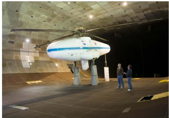
Figure 1. UH-60A Airloads rotor installed on the Large Rotor Test Apparatus (LRTA) in the NFAC 40- by 80-Foot Wind Tunnel.
