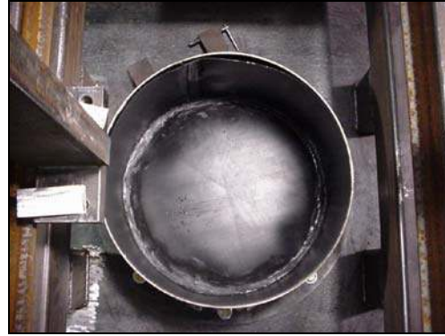
Figure 7. HDPE Cylindrical Liner Inserted in the Water Tank.
