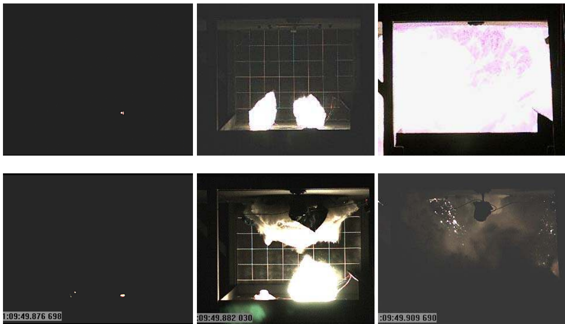
Figure 11. Unsuppressed (top) and Suppressed (bottom) Burns of 4 lbs of MJU 32/38 at Times 0, +5.3, and +33 ms.
