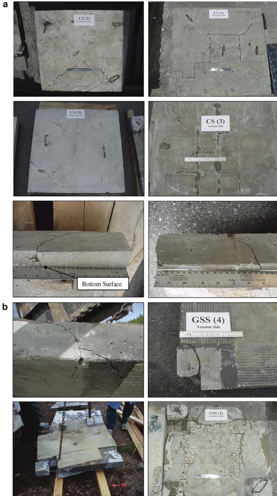
Fig. 7. Typical post-blast observed damage in the test panels (a) panel CS3, (b) panel GSS2.
