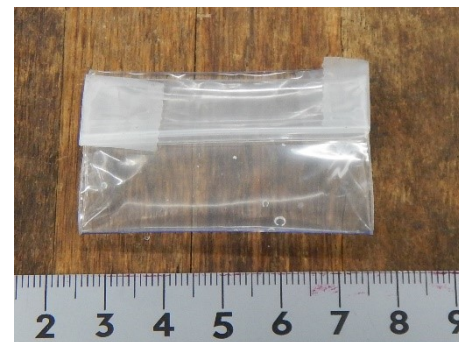
Fig. 2. Water bag for the floor.
