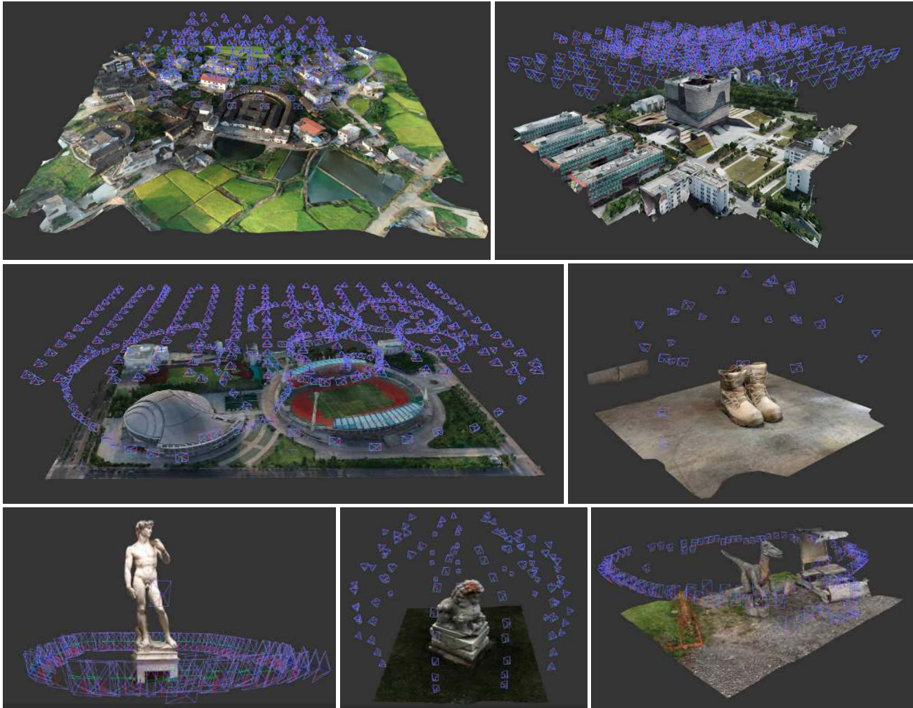
Figure 4: Several textured models with camera trajectories in BlendedMVS dataset. The blue box indicate the camera position in the 3D space. Our dataset contains 113 scenes in total.
