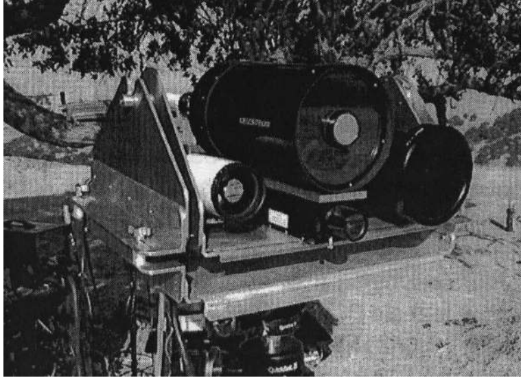
Figure 2.3: Brassboard coherent imaging system. A pulsed laser illuminator with relatively long coherence time is aimed along the optical boresight of a small aperture cassegrain telescope. The system was used to collect a large database of coherently illuminated images of various targets surrounding a mountaintop test range.
