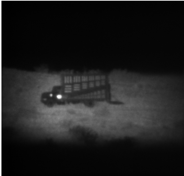
Figure 2.5: Averaged image collected by the coherent vision system. The image was created by averaging 50 spatially registered frames. Registration and averaging is typically required to remove the objectionable effects of coherently formed speckle that is present in each of the individual frames.
