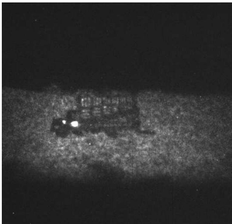
Figure 2.4: Sample image collected by the coherent vision system. The image suffers from heavy degradation due to coherent speckle effects caused by target surface roughness.
