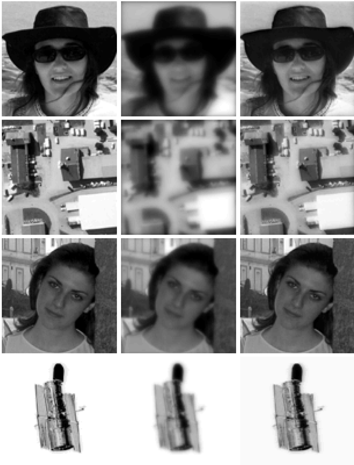
Fig. 7. First column: Source images. Second column: Blurred images. Third column: Restoration results using the QML deconvolution approach.
