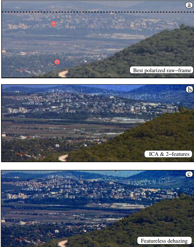
Figure 3. Skyless dehazing of Scene 1 . [a] Best polarized image. The parameters are estimated using the part of the image below the dashed line. The two circles mark buildings which are placed in different depths. [b] Dehazing using ICA and two features. [c] Featureless dehazing. To observe the color effects, please view the paper on the computer monitor.
