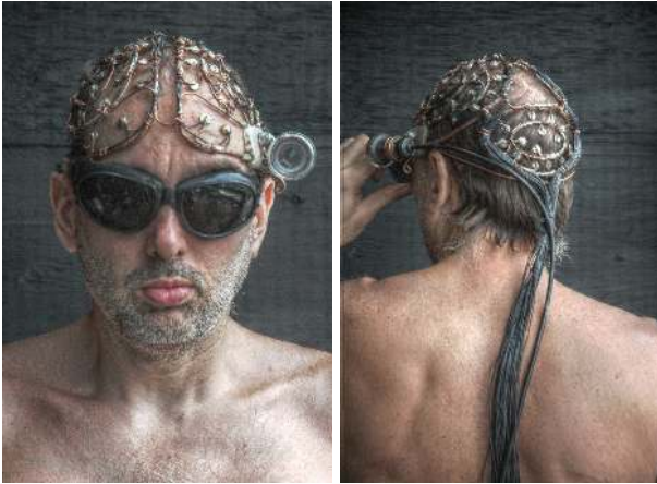
Figure 5: The MindMesh TM BCI (Brain Computer Interface) FPGA mesh-computing architecture has 64 electrodes, so that various items such as the Kinect or more conventional cameras can “plugged into the brain”.
