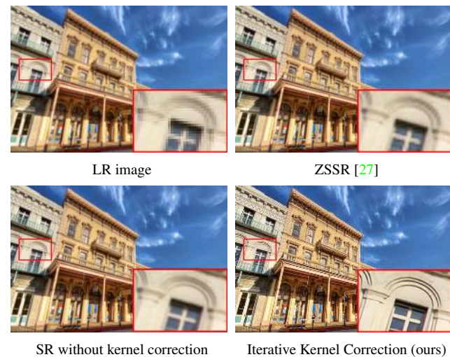
Figure 1. SISR results on image “img_017” with SR factor 4. Before bicubic downsampling, the HR image is blurred by a Gaussian kernel with \sigma = 1.8
