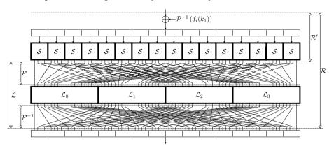
The difference between  $\mathcal{R}$  and  $\mathcal{R}'$  is that in the latter no more diffusion is necessary, therefore the last round ends after the substitution layer. With the software-friendly matrices we have found as described above, the linear layer is defined as follows (cf. Theorem 1 and Appendix G of [2]):
