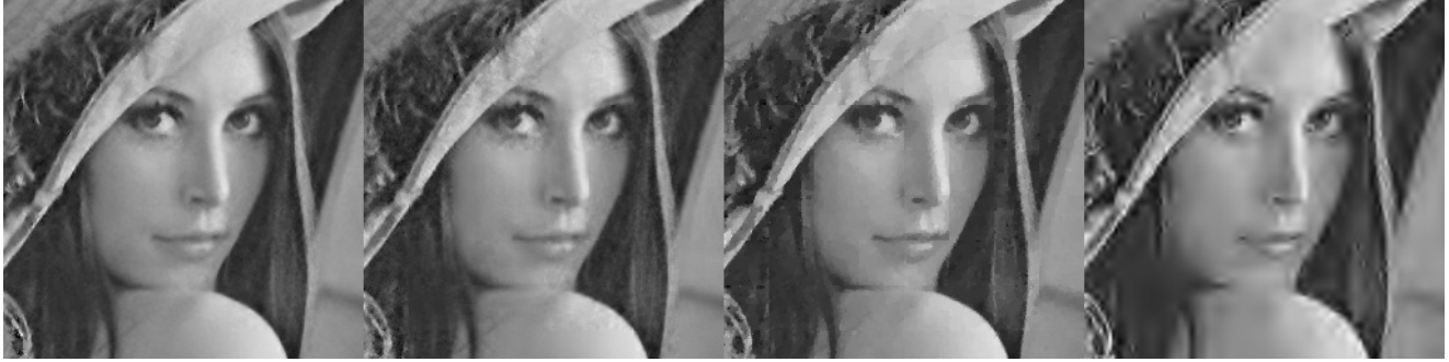
Figure 1: Lenna for M/N = 20\% . Left to right: BCS-SPL-DDWT, PSNR = 31.37 dB; BCS-SPL-DCT, PSNR = 30.45 dB; BCS-TV, PSNR = 30.60 dB; SAMP, PSNR = 28.54 dB.
