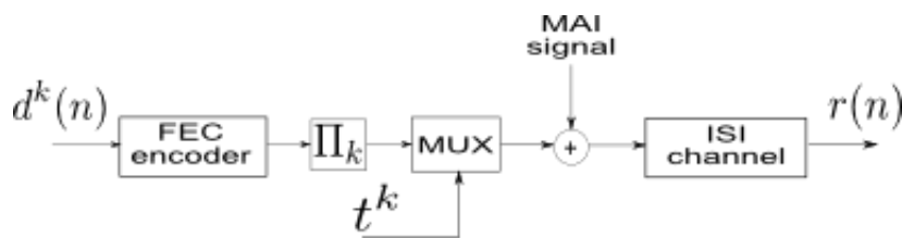
Figure 1. The discrete time block diagram of an IDMA transmitter for user- k .
