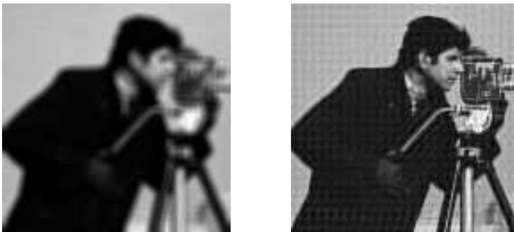
FIG. 4.2. The blurred and noisy image by the average blur (left) and the restored image (right).
