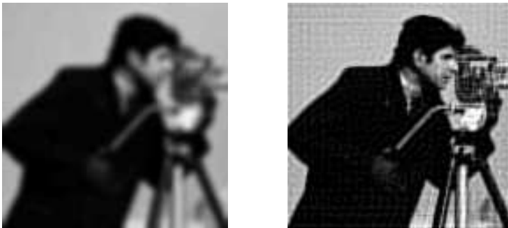
FIG. 4.3. The blurred and noisy image by Gaussian blur (left) and the restored image (right).
