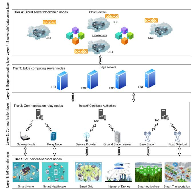
Fig. 8 Blockchain based architecture of IoT
