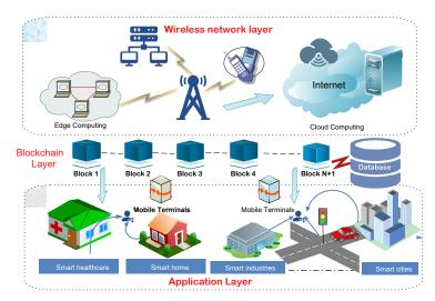
Figure 8. The proposed architecture: enabling blockchain technology for wireless networks.
