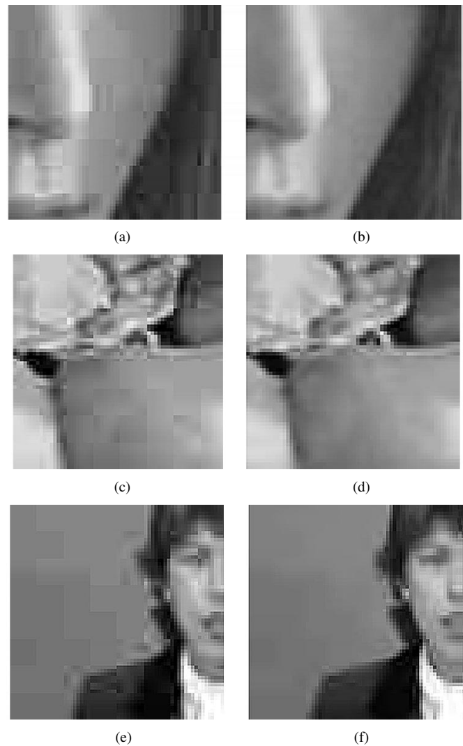
Fig. 10. (a) Portion of the JPEG coded "Lena" image at 0.2989 bpp. (b) Reduction of blocking artifacts with the proposed method at 0.2989 bpp. (c) Portion of the JPEG coded "Peppers" image at 0.3137 bpp. (d) Reduction of blocking artifacts with the proposed method at 0.3137 bpp. (e) Portion of the JPEG coded "Claire" image at 0.3779 bpp. (f) Reduction of blocking artifacts with the proposed method at 0.3779 bpp.
