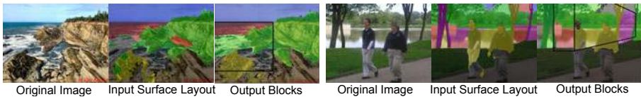
Fig. 10. Failure Cases: We fail to recover proper geometry when [8] is confident about the wrong predictions. Our approach also hallucinates blocks whenever there is a possible convex corner. For example, in the second image the wrong surface layout predicts a false corner and our approach strengthens this volumetric interpretation.
