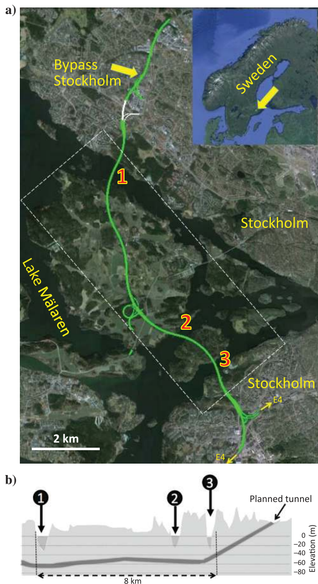
Figure 3. (a) The Bypass Stockholm project plan. The green line is the planned track, and the frame on the top-right corner shows the location of the study area in Sweden. (b) Cross section of part of the planned tunnels (marked with the dashed white box in panel [a]) below Lake Mälaren. Sites 1, 2, and 3 are where the case study was conducted.
