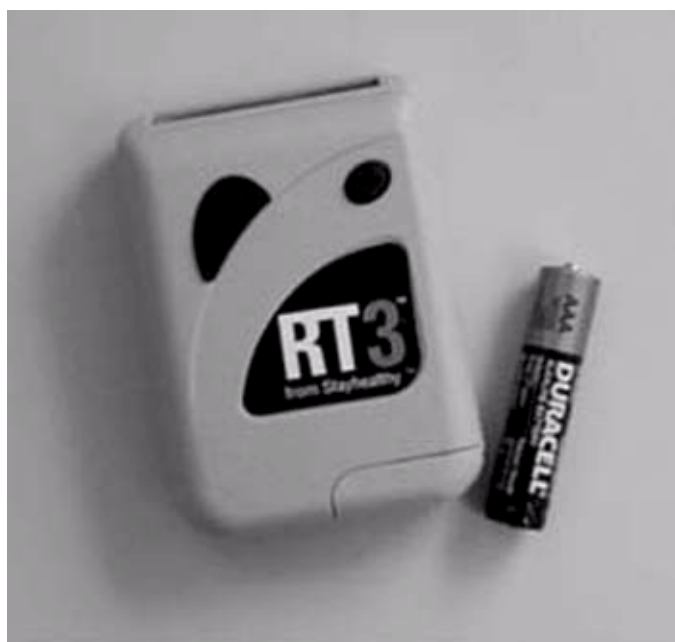
Figure 5. RT3 ® accelerometer from StayHealthy ® , next to AAA battery to demonstrate scale. Buttons are event markers, useful during analysis for matching vector magnitude units with diary entries.
