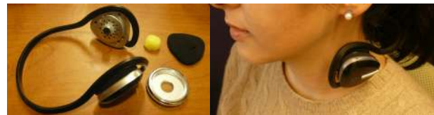
Figure 1. The BodyScope prototype. It consists of a Bluetooth headset, a microphone (embedded in the headset), and the chestpiece of a stethoscope.
