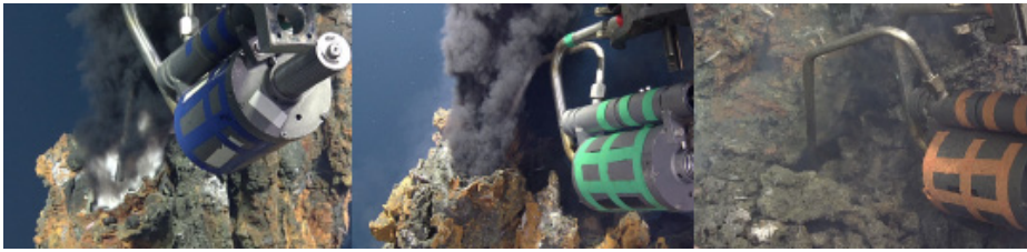
Figure 1. Photographs of types of fluid emission. Left to right: boiling hydrothermal fluid, focused flow fluid, diffuse flow fluid. Snorkel nozzle is ½" diameter.
