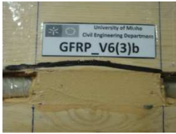
GS – Glulam shear failure
