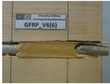
GAI – Glulam/adhesive interfacial sliding
