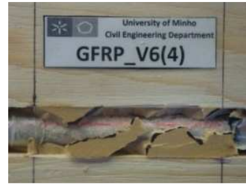
FAI+SPL – FRP/adhesive interfacial sliding + adhesive splitting
