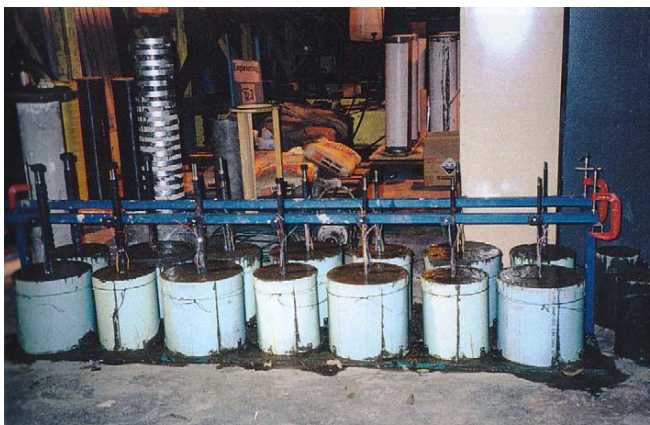
Fig. (4). Casting the specimens.
