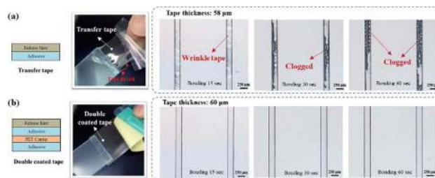
Fig. 3 Microchannel bonding with a (a) transfer tape and (b) double-coated tape under different bonding conditions.
