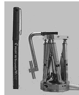
Fig. 2. Photograph of the MARS. The robot is shown with an angled drill guide mounted on its upper base.
